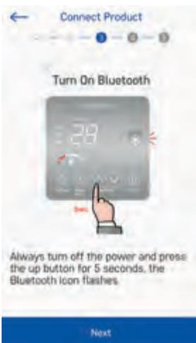
6. Turn the heater power off and press the up button for 5 seconds. Then the bluetooth icon flashes. Press NEXT button in the application.
