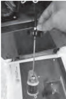
The fuel filter is located in the heater tank. The filter replacement cycle is recommended for 6 months. (Depending on oil quality.)
