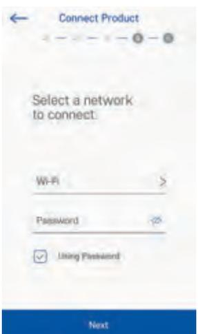
8. Choose your Wi-Fi network by pressing the Wi-Fi selection. After choosing your Wi-Fi, fill in the correct Wi-Fi password in the password field. Press NEXT to connect your heater to your own Wi-Fi.
