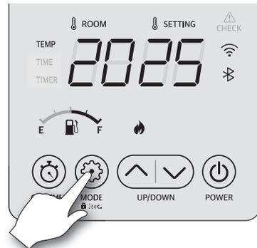
3. The temperature can be adjusted with the arrow buttons.
