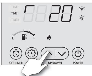
4. The operating time can be set between 10 and 55 minutes, or the heater can be set to run continuously. Once the operating cycle ends, the heater always suspends operation for five (5) minutes. Two lines (- -) are shown on the display alongside the operating time to indicate the pause.
