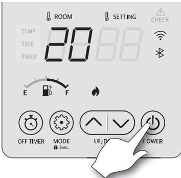
2. The corresponding signal light is on when thermostat operation is selected. To switch from thermostat operation to timer operation, press the MODE button.
