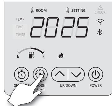
3. When timer operation is on, a light ring is shown on the left. The set operating time (in minutes) is displayed on the right. Select the desired operating time with the arrow buttons. The selected time flashes on the display. If the arrow buttons are not pressed for three (3) seconds, the time setting shown on the screen is activated.
