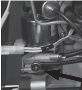
If the heater's fuel pump sounds exceptionally loud and the heater does not run properly, the probable cause is air in the fuel system.
